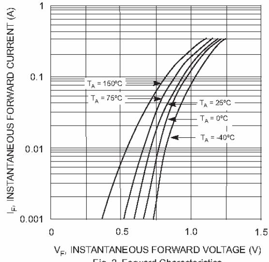
Fig. 2 Forward Characteristics
