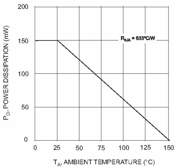
Fig. 1 Derating Curve
